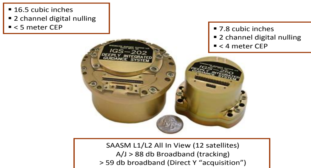
Figure 18. IGS-202 and IGS-250 Deeply Integrated Guidance Systems [20]
